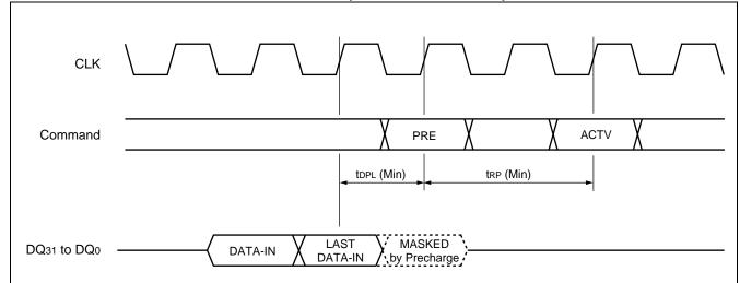
Note: The precharge command (PRE) should only be issued after the topl of final data input is satisfied. PRE means 'PRE' or 'PALL'.
