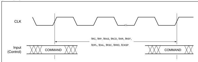
Note: These parameters are a limit value of the rising edge of the clock from one command input to next input. toke is the latency value from the rising edge of CKE.
