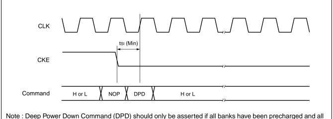
Note: Deep Power Down Command (DPD) should only be asserted if all banks have been precharged and all outputs are in High-Z.
